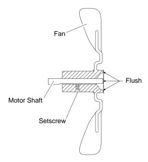
Figure 22 - Fan Cross Section
